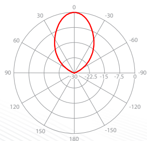
V/H - Port Pattern Azimuth 5.6 GHz
