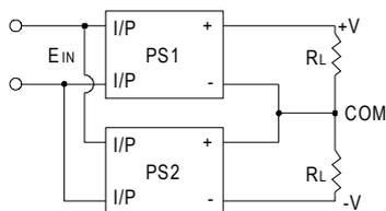
2. Increase the output voltage (current does not change). Because RSD-200 series have no reverse blocking diode in the unit, you should add an external blocking diode to prevent the damage of every unit while starting up. The voltage rating of the external diode should be larger than  $V1+V2$  (as shown as below).
